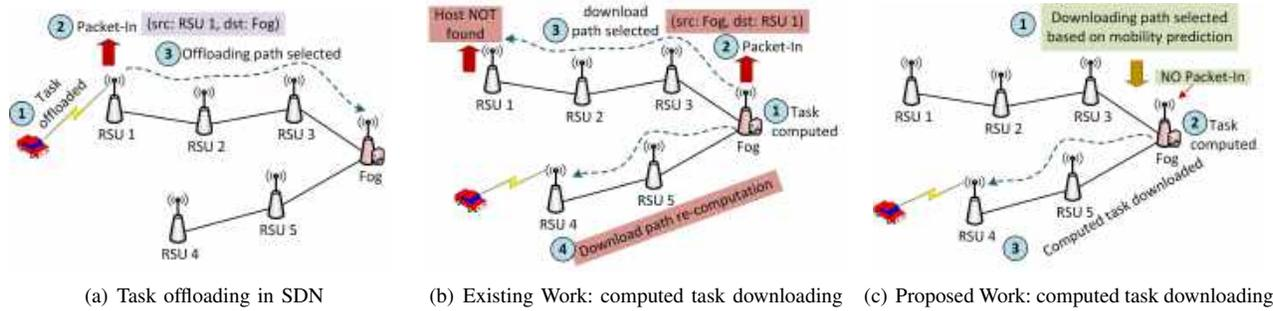
Fig. 1: Motivating scenario: a) task offloading in software-defined vehicular network; b) Issues due to mobility of vehicles and reactive approach; c) Proactive scheme (proposed)
