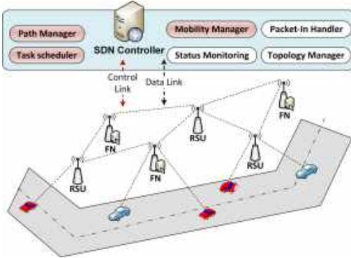
Fig. 2: Software-defined architecture of fog-based VANET
