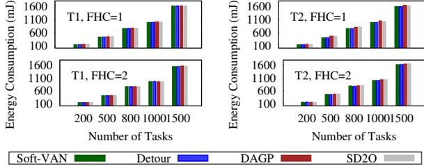
Fig. 6: Energy consumption per vehicle with different tasks
