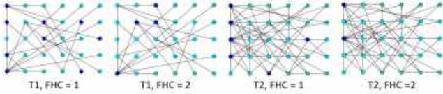
Fig. 4: Network topology and fog node selection using different hop-count (fog nodes in blue color)
